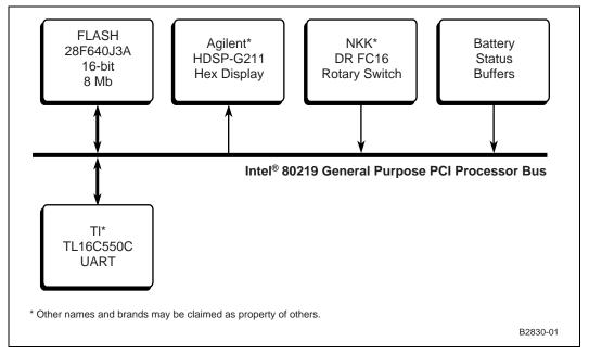
The devices on the bus include Flash ROM, UART, HEX display, and rotary switch.
